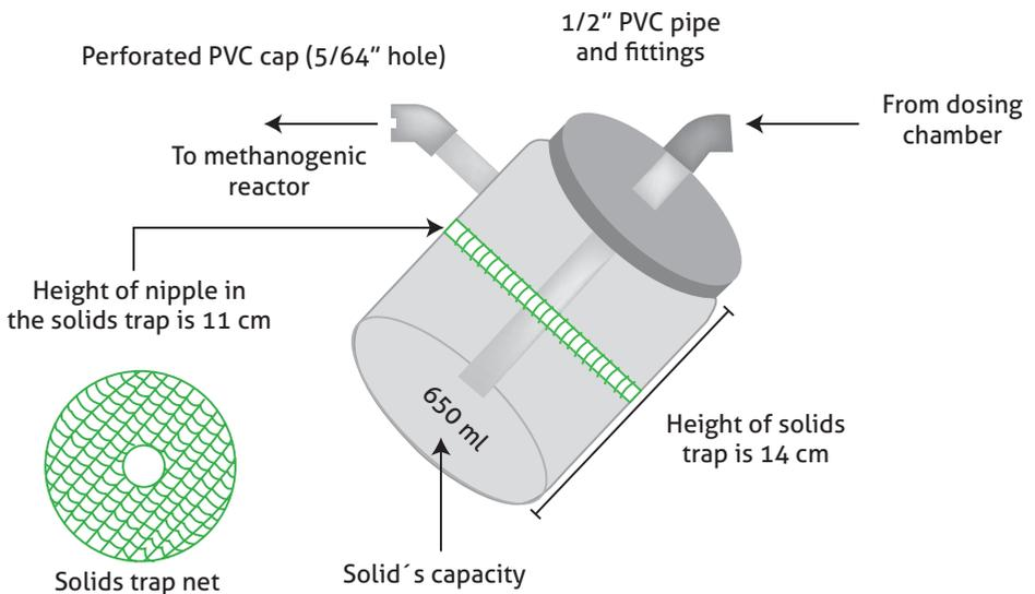
Figure 45. Diagram of solids trap.
