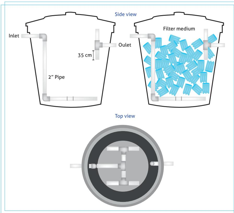
Figure 29. Characteristics of anaerobic filters.
