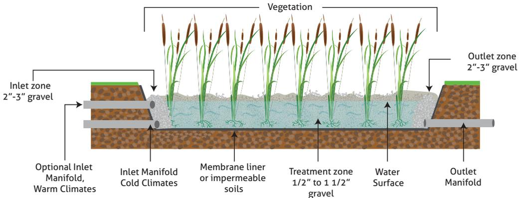
Figure 31. Constructed subsurface flow wetland diagram (Source: EPA, 2000).
