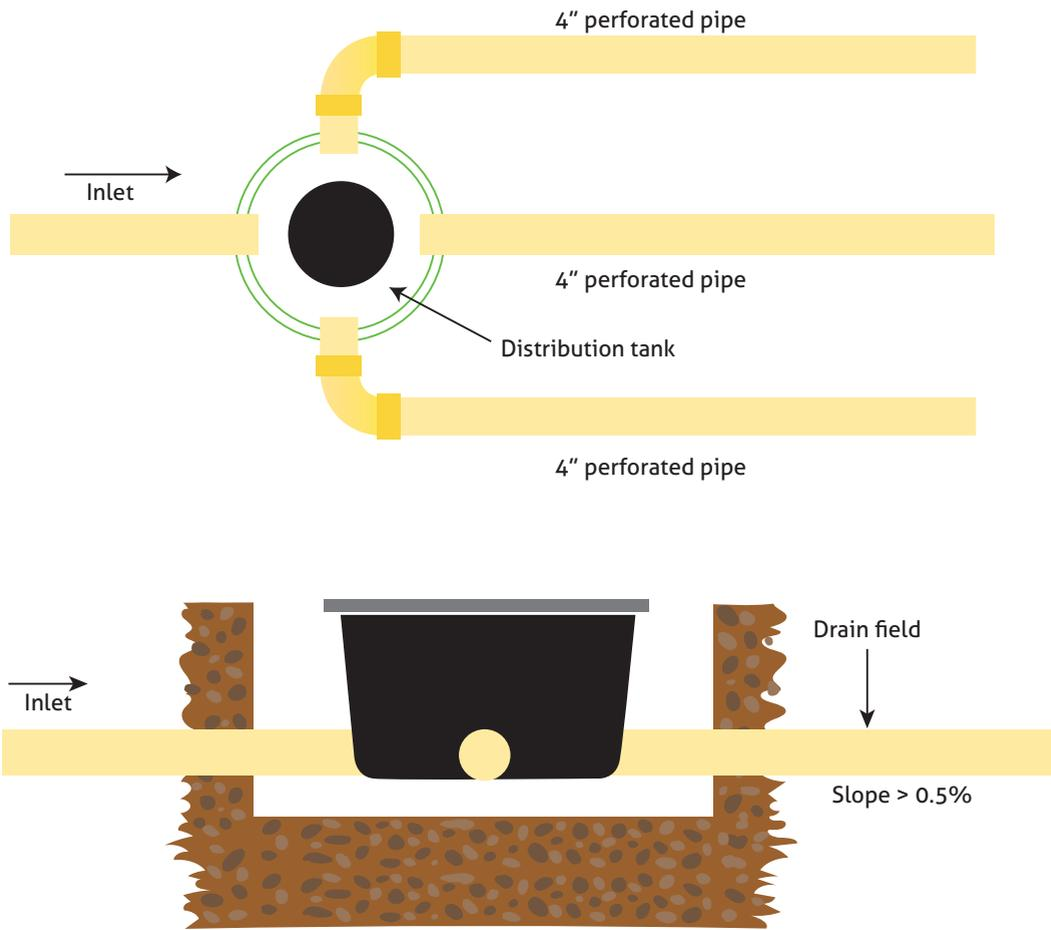
Figure 37. Distribution tank diagram.
