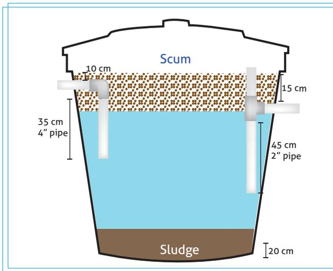
Figure 20. Details of septic tank.
