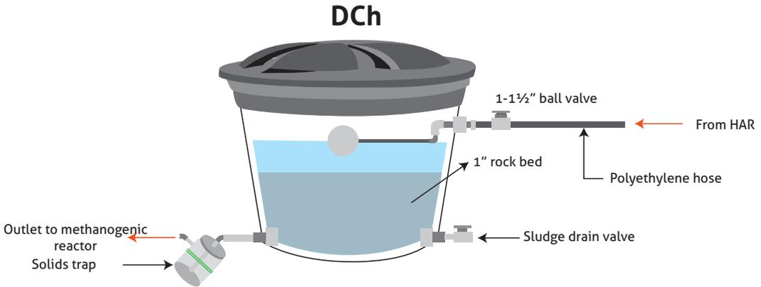
Figure 46. Location of solids trap after the dosing chamber.
