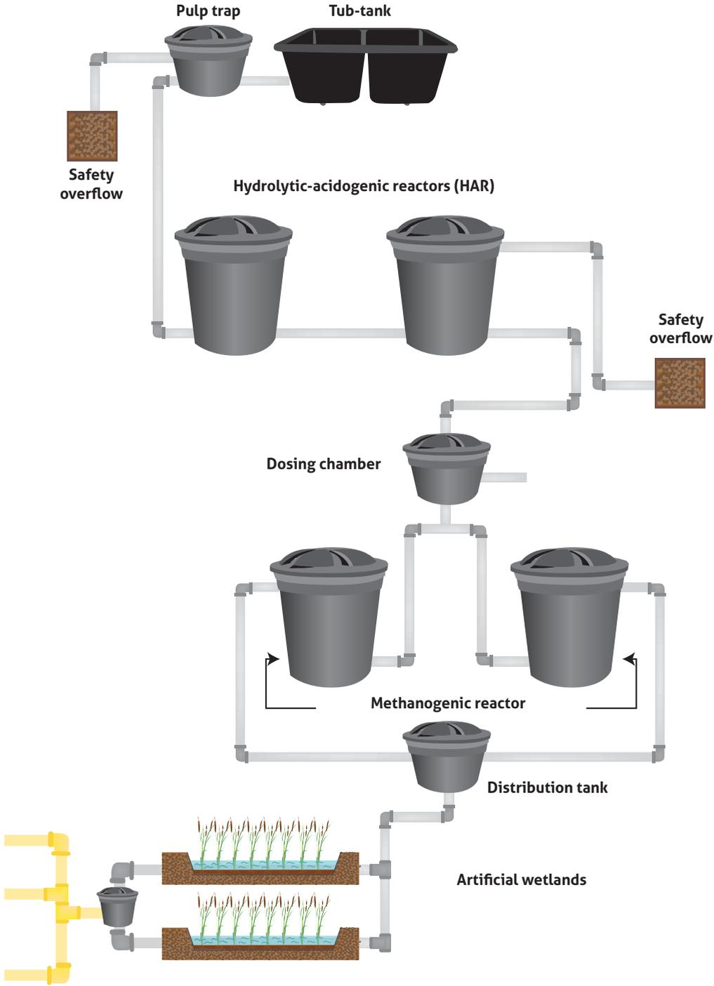
Figure 41. Modular Anaerobic Treatment System Diagram.
