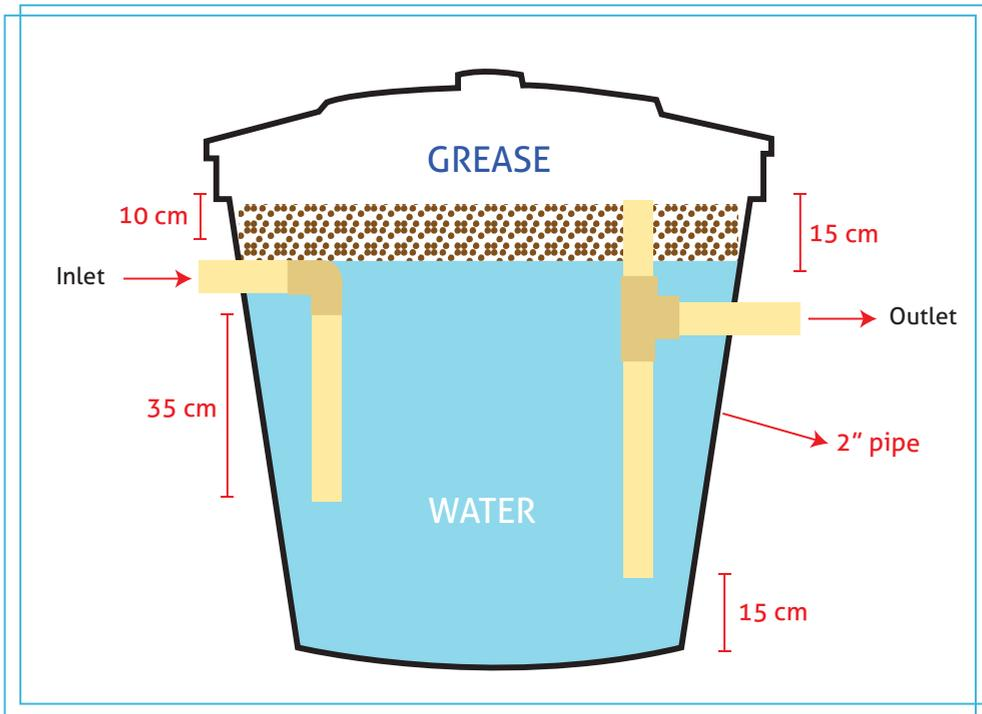
Figure 17. Grease trap.
