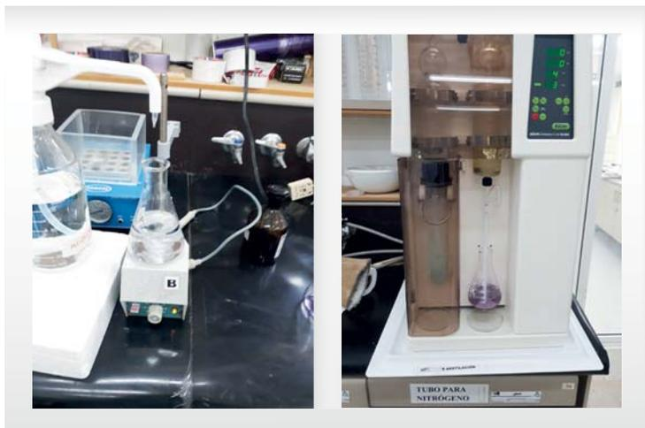
Figure 7. Determination of nitrogen by the Kjeldahl method.
