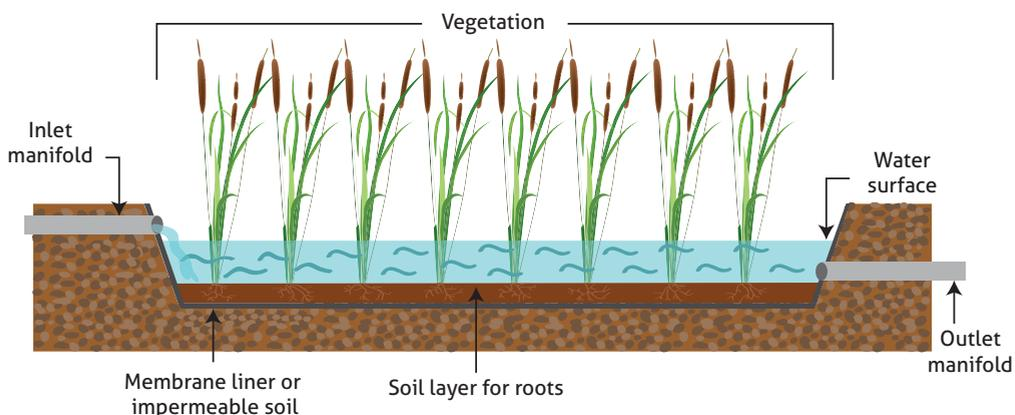
Figure 30. Free water surface wetland diagram (Source: EPA, 2000).
