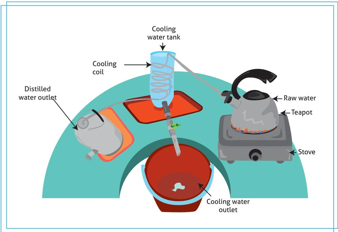
Figure 12. Distillation system with teapot.
