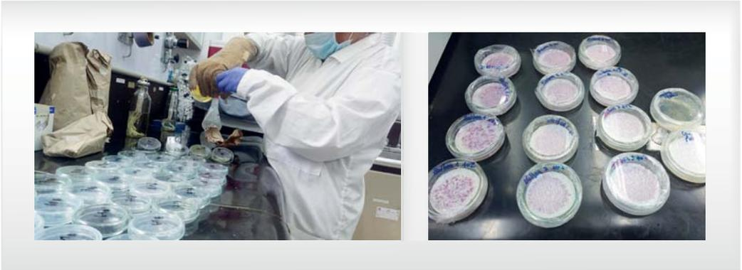
Figure 10. Determination of total and fecal coliforms.
