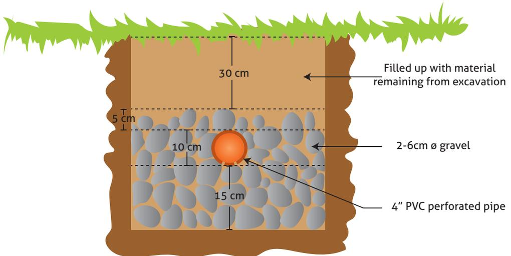
Figure 39. Diagram of one of the drain trenches.
