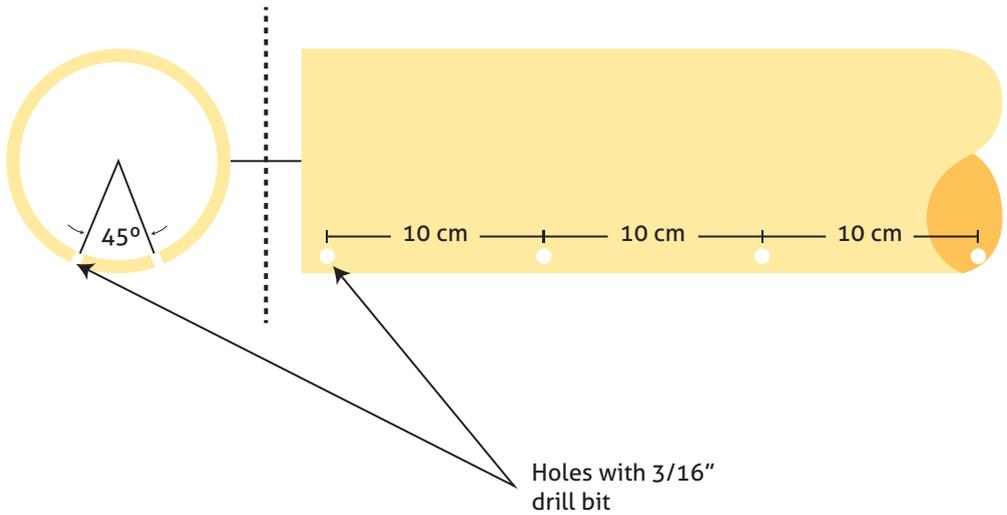
Figure 38. Diagram of holes in distribution pipes.
