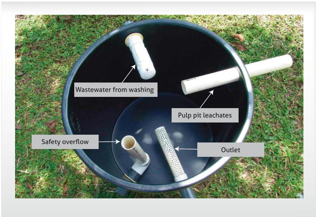
Figure 42. Pulp trap diagram.
