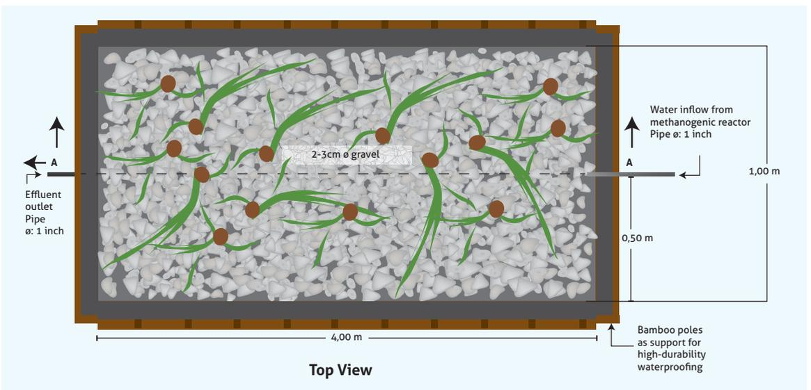
Figure 35. Diagram of wetlands built in IWM Project.
