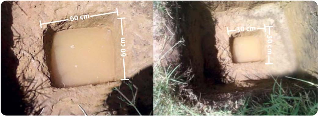
Figure 36. Percolation tests for design of drain fields.
