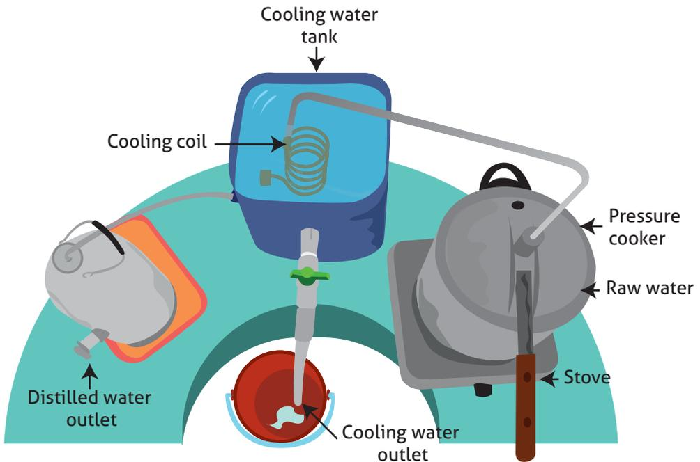
Figure 11. Distillation system with pressure cooker.
