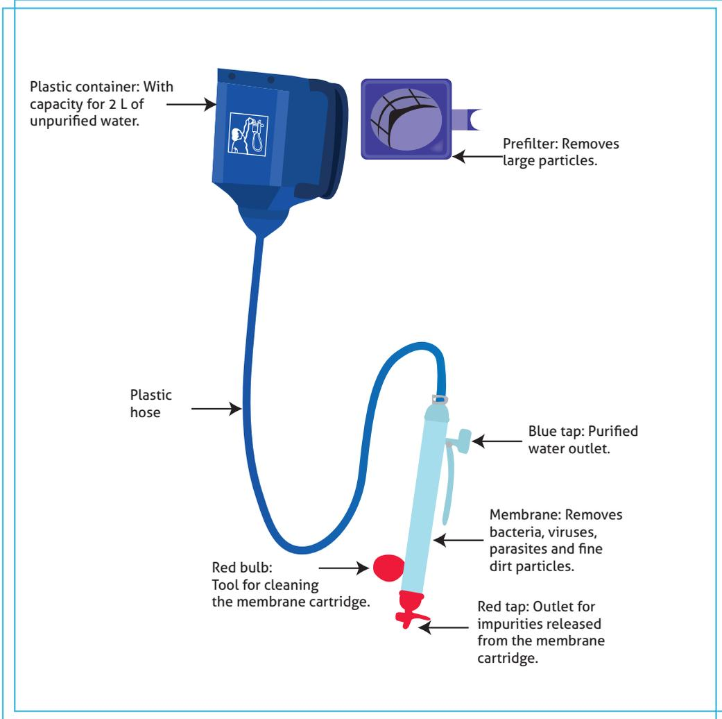
Figure 13. Nanofiltration system (Source: [www.iwanagreen.com](http://www.iwanagreen.com)).
