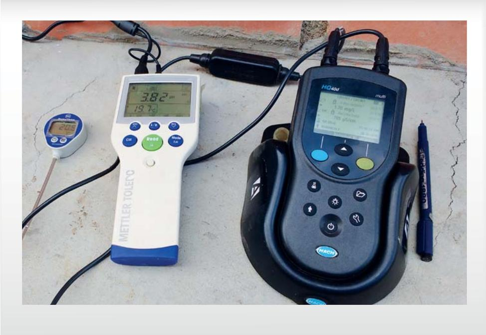
Figure 9. Equipment for determination of pH.
