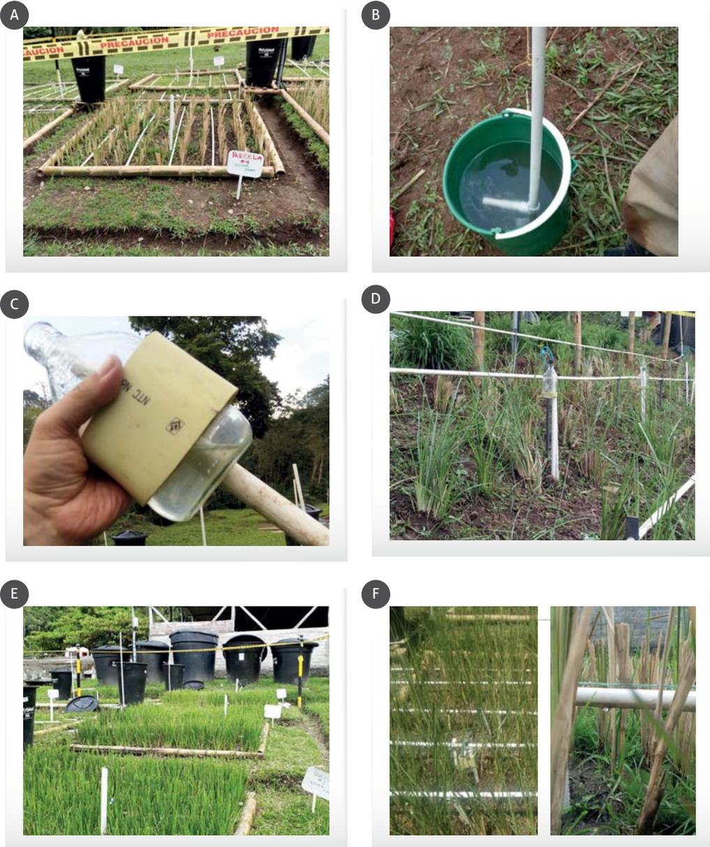
Figure 51. (a) The plots before the experiment; (b) Horizontal suction lysimeter; (c) Sampling container and irrigation system; (d) Leveling of irrigation pipes; (e) Plots at completion of the experiment; (f) Flow distribution system.
